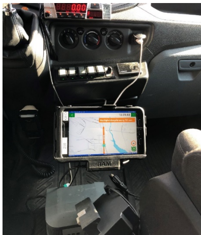
Figure 1: Installation of the tablet in the vehicle's central console
