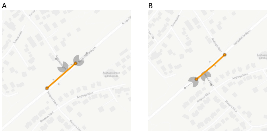
Figure 5: Assigned trigger signals in SkanTech's geofence zone designer interface for two road segments leading in opposite directions
