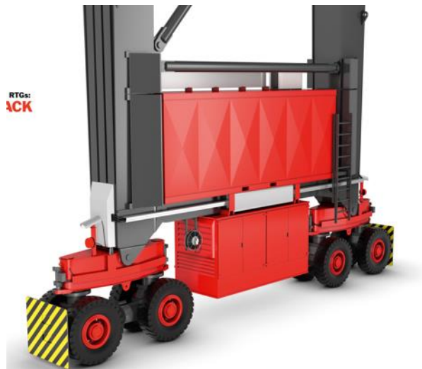
Figure 4.2.1. Hybrid RTG with rechargeable power pack.
