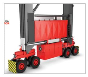
Figure 8.4. Hybrid RTG with rechargeable power pack Source: www.moveitmagazine.com/2019/03/22.
