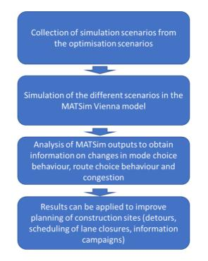
Figure 11 Approach to apply an agent based MATSim model for the planning of construction sites.
