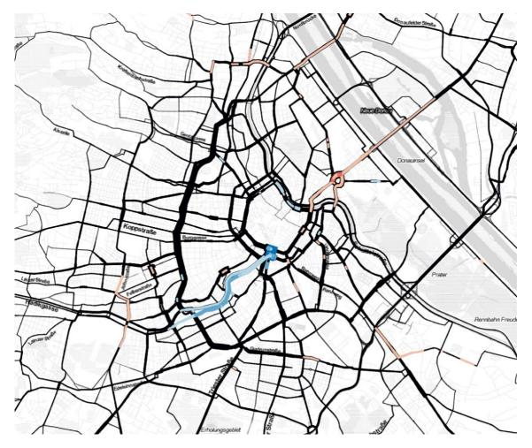
Figure 10 Estimated link flow volumes in the road network in March 2019 (before the construction work) and significant increase (red) and decrease (blue) during the construction work in July 2019.
