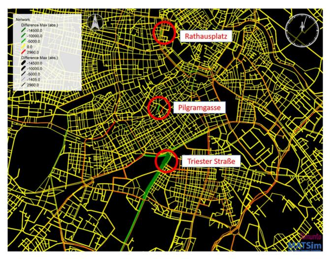
Figure 13 Difference in car counts on the links between the base line scenario and scenario 2.
