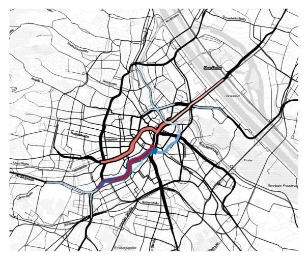
Figure 9 Estimated link flow volumes in the public transportation network in March 2019 (before the construction works) and significant increase (red) and decrease (blue) during the construction work in July 2019.
